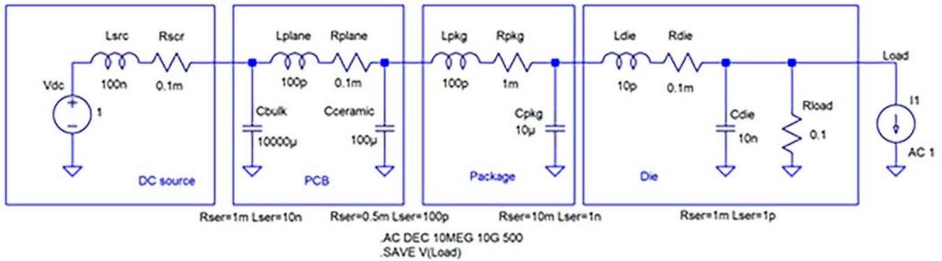
Figure 2: LTSPICE schematics of a simple point-of-load PDN.
