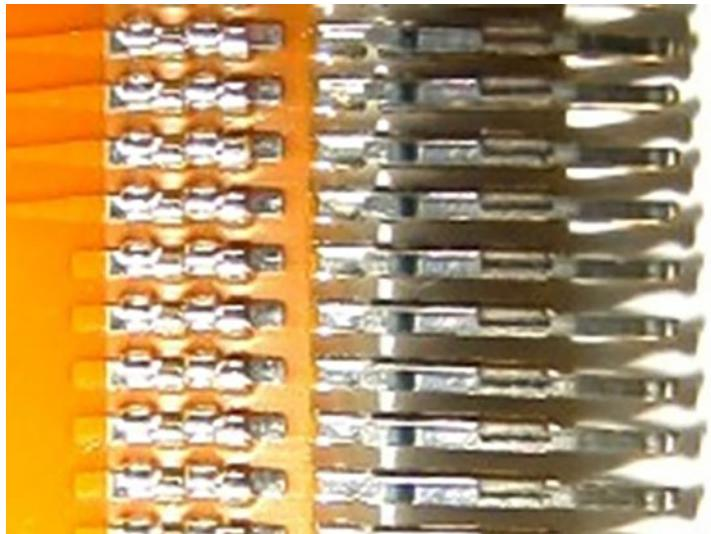
Figure 2: Pierce type connector for flex to rigid header.
