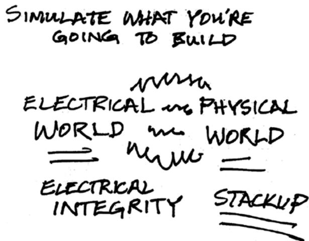
Figure 2: The fundamental reason for signal-integrity or power-integrity simulation is to predict the negative impact that the physical world has on the electrical world, and to mitigate or prevent the negative effects proactively. (Artwork by yours truly.)
