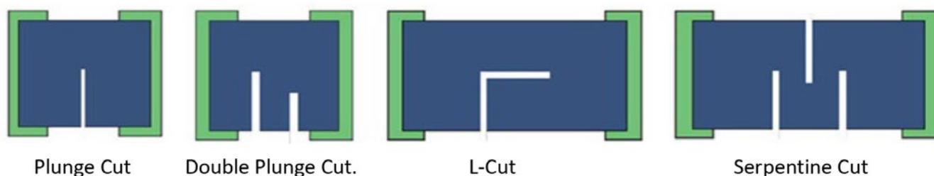
Figure 2: Laser trim variations for thick film resistor elements. (Trim examples courtesy of PPI Systems)
