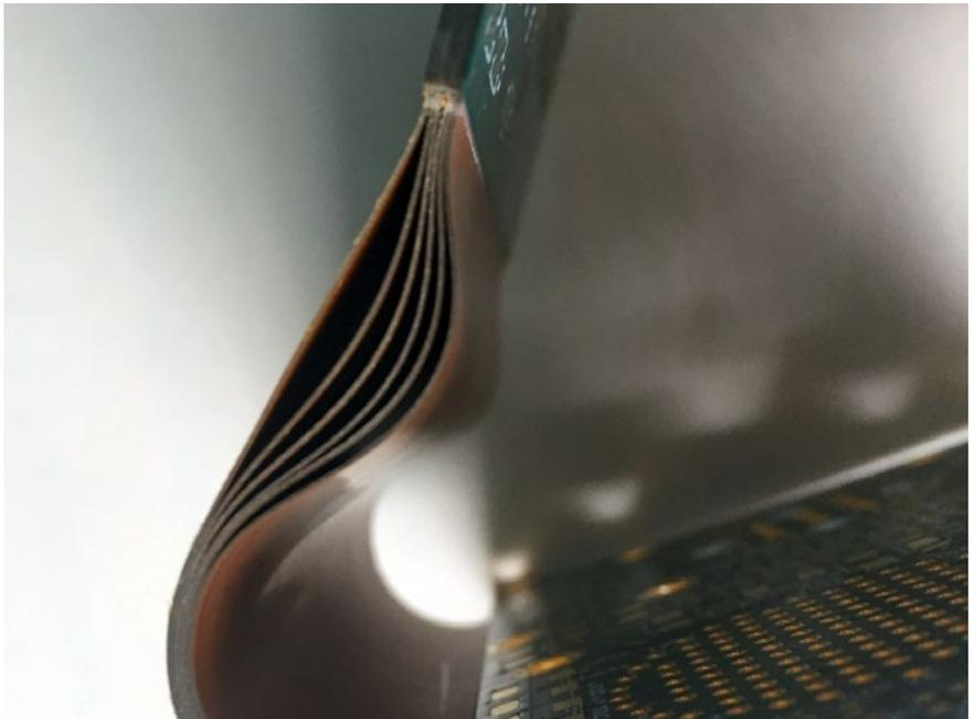
Figure 3: Completed PCB flex belts separated.
