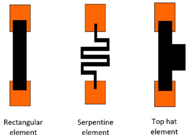
Figure 1: Thick film resistor pattern variations.
