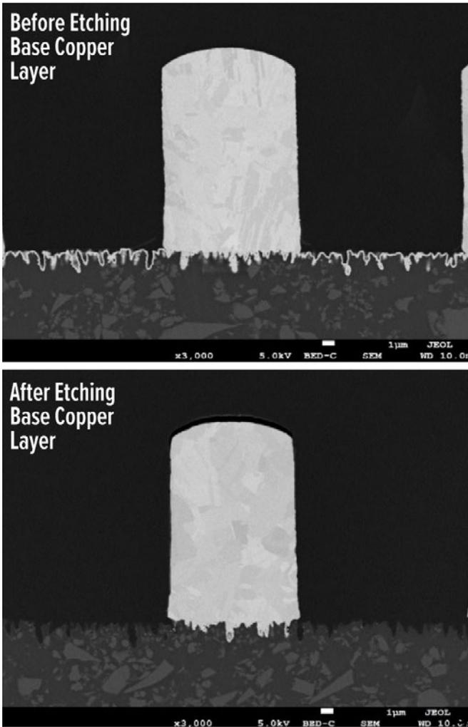
Figure 2: Before and after etching the base copper layer. (Images courtesy of MEC Corporation)
