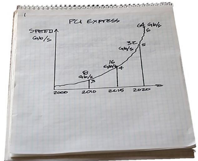
Figure 1: Interconnect speed increases in gigabits per second (Gbps) from 2000. (Artwork by yours truly.)
