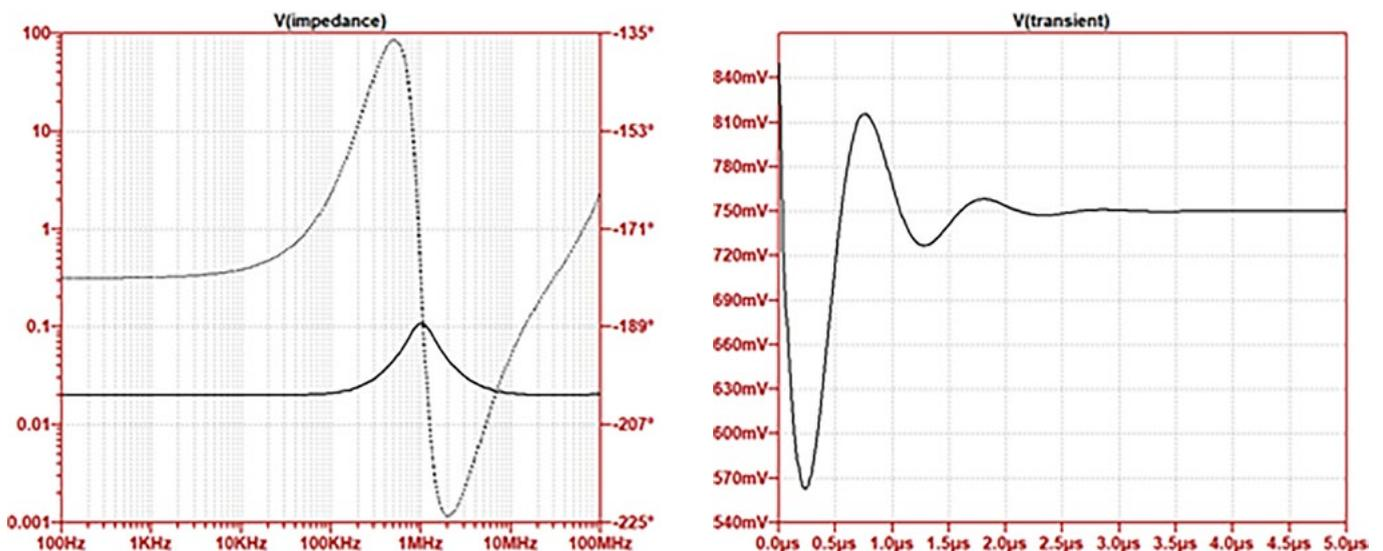
Figure 5: Impedance profile (on the left) and transient response (on the right) of the circuit in Figure 2 when we change the series inductance from 1 nH to 10 nH.
