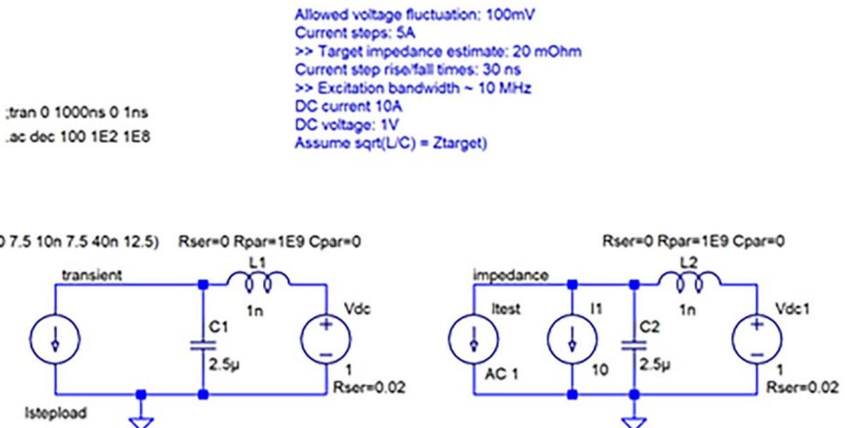
Figure 3: LTSPICE schematics for a one-stage L-C PDN circuit with matched source and load.
