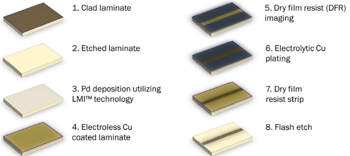
Figure 1: A-SAP™ process flow diagram.
