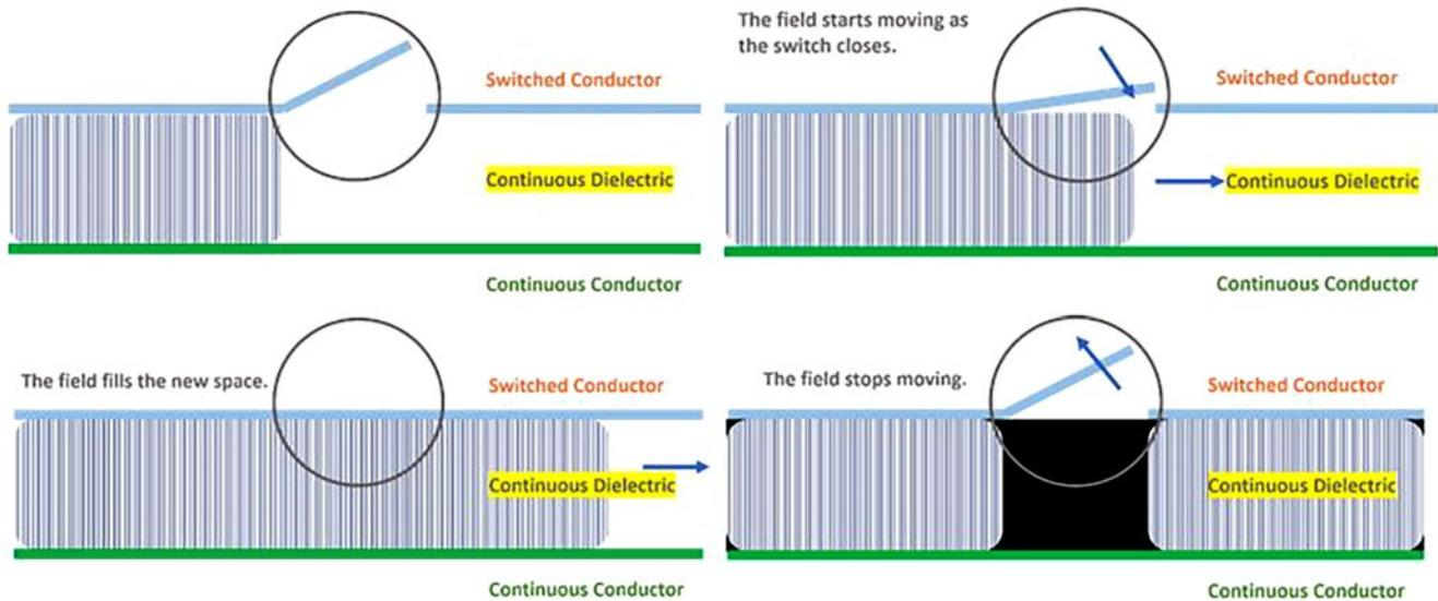
Figure 3: Images depicting the movement of an EM field as a switch closes. There are only three things that you can do with EM fields: Store them, move them, or convert them into kinetic energy.
