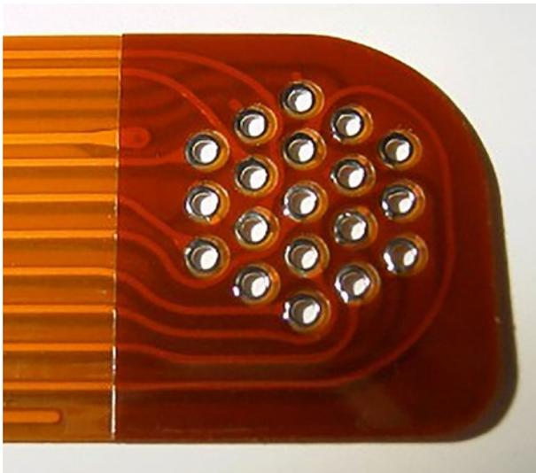
Figure 1: Reinforced flex for soldering to military connector.
