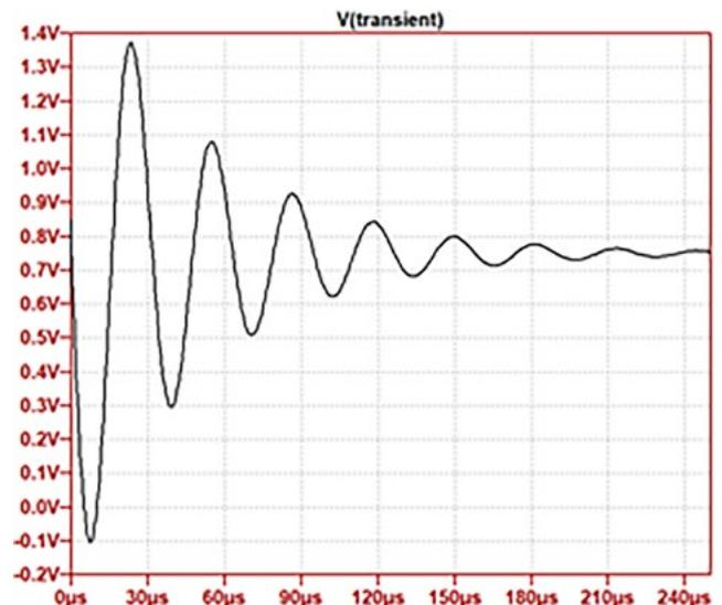
Figure 7: Impedance profile (on the left) and transient response (on the right) of the circuit in Figure 6.
