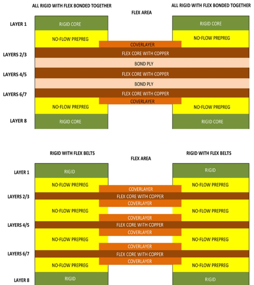
Figure 2: Bonded vs. unbonded flex areas.
