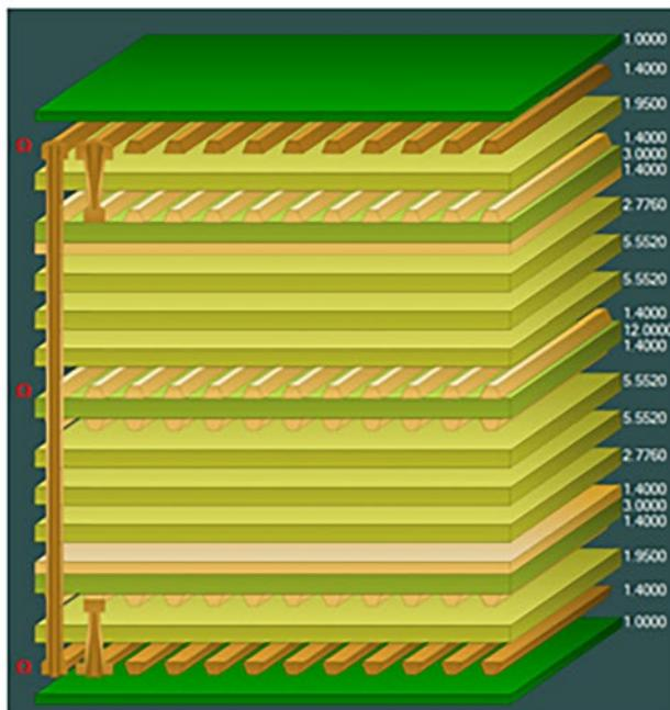
Figure 4: Traditional glass cloth/epoxy resin weave. (Source: Ventec International Group)
