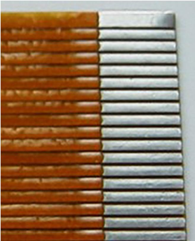
Figure 3: Finger flex connector for insertion into connector on rigid PCB.
