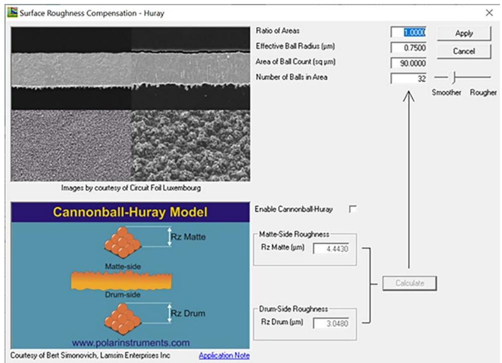
Figure 7: Modeling roughness with SEM or Cannonball model.
