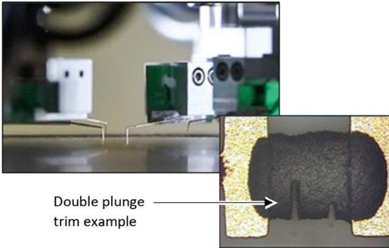
Figure 3: Laser trim system equipped with flying probe contactors. (Source: PPI Systems)
