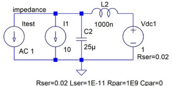
Figure 6: The circuit of Figure 3 with 1000 nH inductance and 25 mF capacitance.
