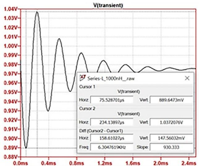
Figure 9: Impedance profile (left) and transient response (right) after we decrease AC losses by tenfold.
