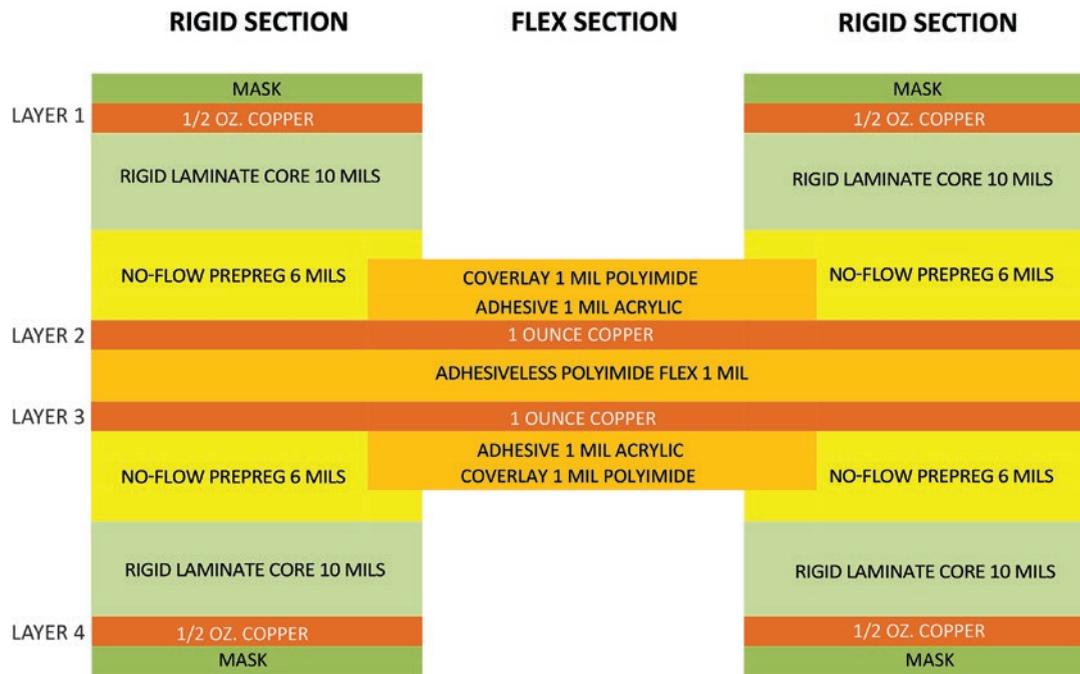
Figure 1: Example of four-layer flex construction.
