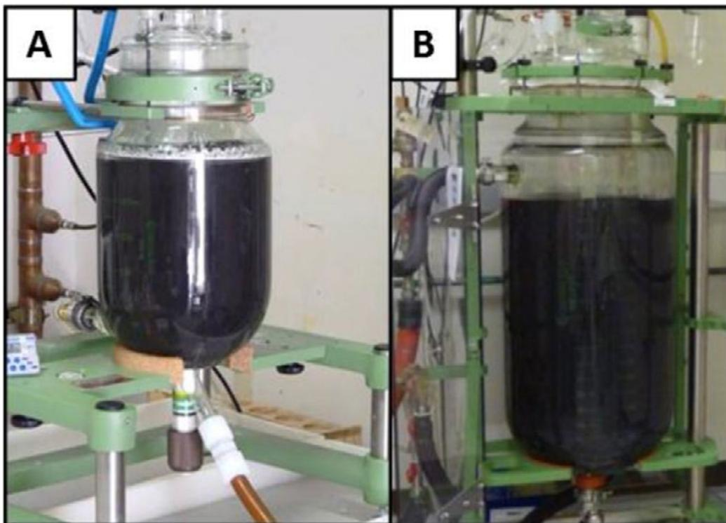
Figure 3: Nanocopper reaction at the 5 L scale (A) and 80 L scale (B).
