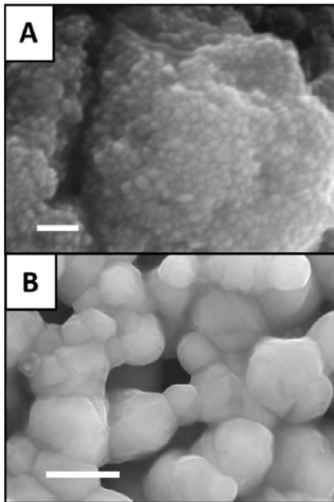
Figure 4: SEM micrographs of copper nanoparticles isolated from the synthesis (A) and material after fusing at 210°C for four minutes (B). The scale bars represent 100 nm and 500 nm for panels A and B, respectively.
