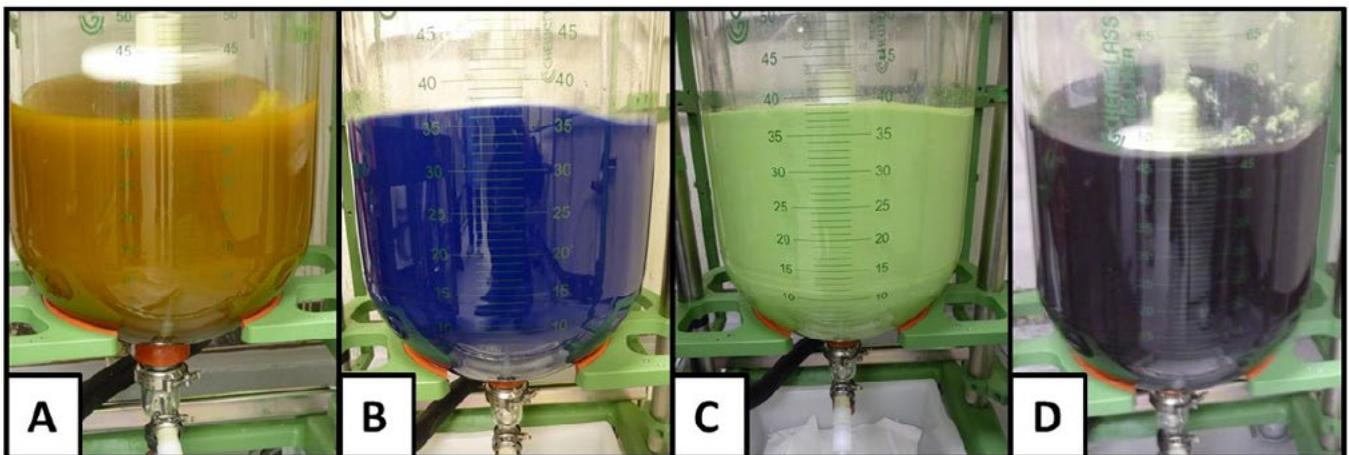
Figure 2: Reaction progression from a soluble copper salt (A-C) to reduction to copper nanoparticles (D).
