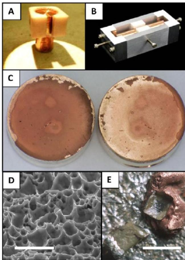
Figure 5: A–E) A) A single copper bar used for tensile testing is nested within a Teflon collar. B) A tensile specimen loaded in a fixture ready for fusion. C) Photograph of a fracture surface following tensile testing. D) SEM image of a fracture surface after tensile testing. The scale bar represents 5  $\mu\text{m}$ . E) A surface mount resistor bonded to a Sn surface with nanocopper. The resistor failed in the ceramic rather than the nanocopper when stressed. The scale bar represents 1 mm.
