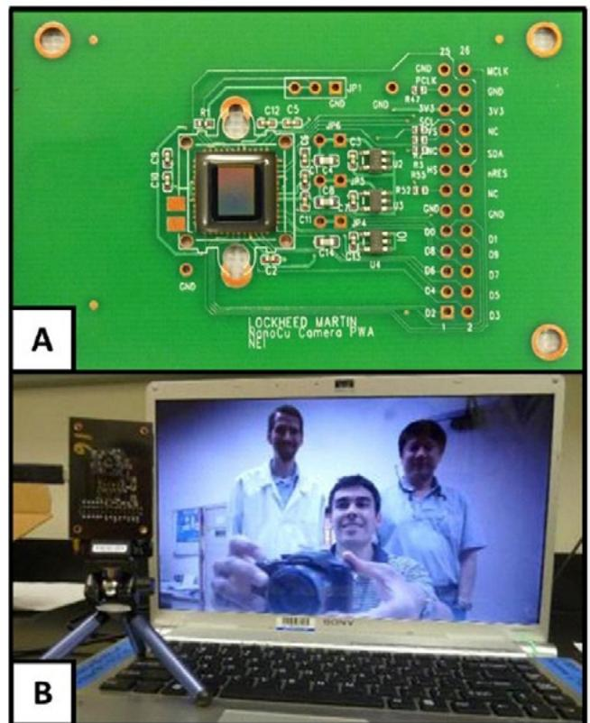
Figure 6: A) Photograph of a camera board populated with all surface mount components. B) Demonstration of fully functional camera board using only nanocopper.
