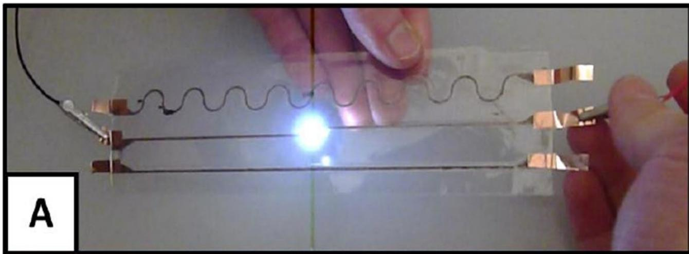
Figure 7: Photograph of flexible LED circuits with stencil printed nanocopper traces.
